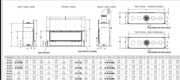
Dimensions are in inches and millimeters. Product information is not complete and is subject to change without notice. Product installation must adhere strictly to instructions shipped with product. We recommend measuring individual units at installation. Assumes the use of 1/2" sheetrock. NOTE: Combustible material should not cover the face. Make sure you do NOT cover the decorative door opening.
